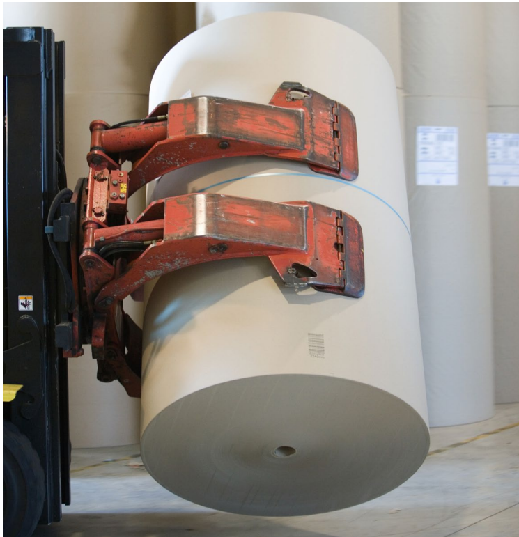
Forklift transporting roll of paper in warehouse. Source: Getty Images
